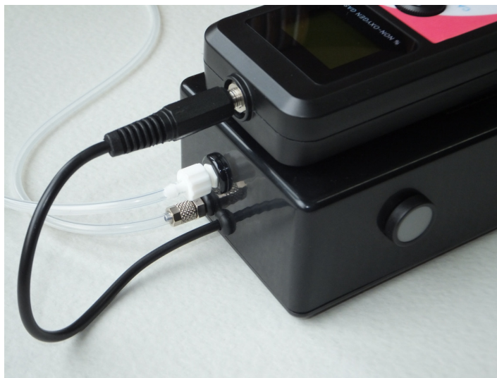
Fig.4 – Connecting the pump box to the analyser
