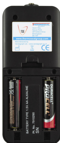
Fig.2 – Battery location in the NM-Argon Analyser
