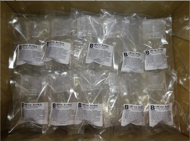
While packing the sensors perform occasional spot checks on random sensors throughout the batch to ensure the serial number and date code on the sensor label matches the bag label. Take special care to check that each bag is properly sealed, there is a blue heat sealer located on the QA shelf which may be used to go over any inadequate seals.
