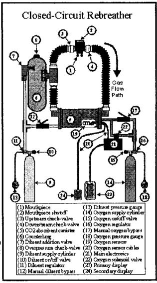
open-circuit system at the operating depth of the dive. This supply is used to maintain system volume during excursions to depths where the volume of gas in the breathing loop is compressed. In some rebreathers the diluent is also used for the emergency open-circuit bailout gas supply in the event of a total system failure of the rebreather apparatus.
