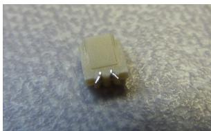
5) Place the JST connector on to the PCB, ensuring that the connector contacts align with the contacts of the PCB.
