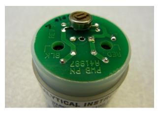
4) Splay the solder contacts to around a 30° angle.
