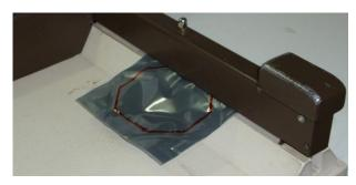
3. Fill the transducer cushion with water, leaving as little air in the cushion as possible, and seal.
