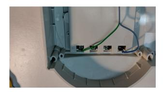
Connect the 2 pin M22 connector to the 2 pin connector on the PCB.
