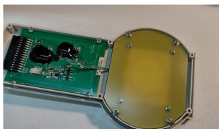
Connect the transducer assembly to the PCB using the 3 pin connector.
