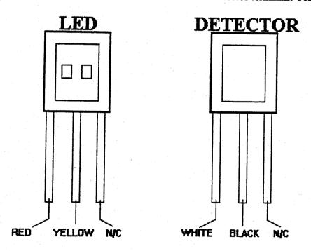
9. Inspect finger pads (item 5 & 6) for damage or cracks. Replace finger pads if damaged or cracked. Slide the LED into the top pad and silicone (item 23) into place. Slide the Detector into the bottom pad and silicone (item 23) into place. Let silicone dry.
