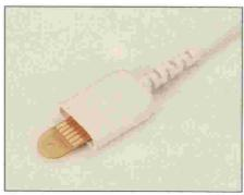
CT-7055A FLEX CIRCUIT BOARD MOLDED TO PIGTAIL
